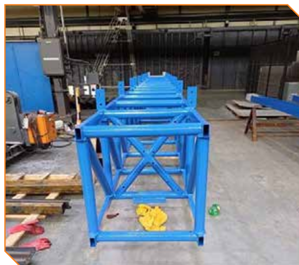
Figure 22: Painted gantry structure ready for assembly outside NECSA
