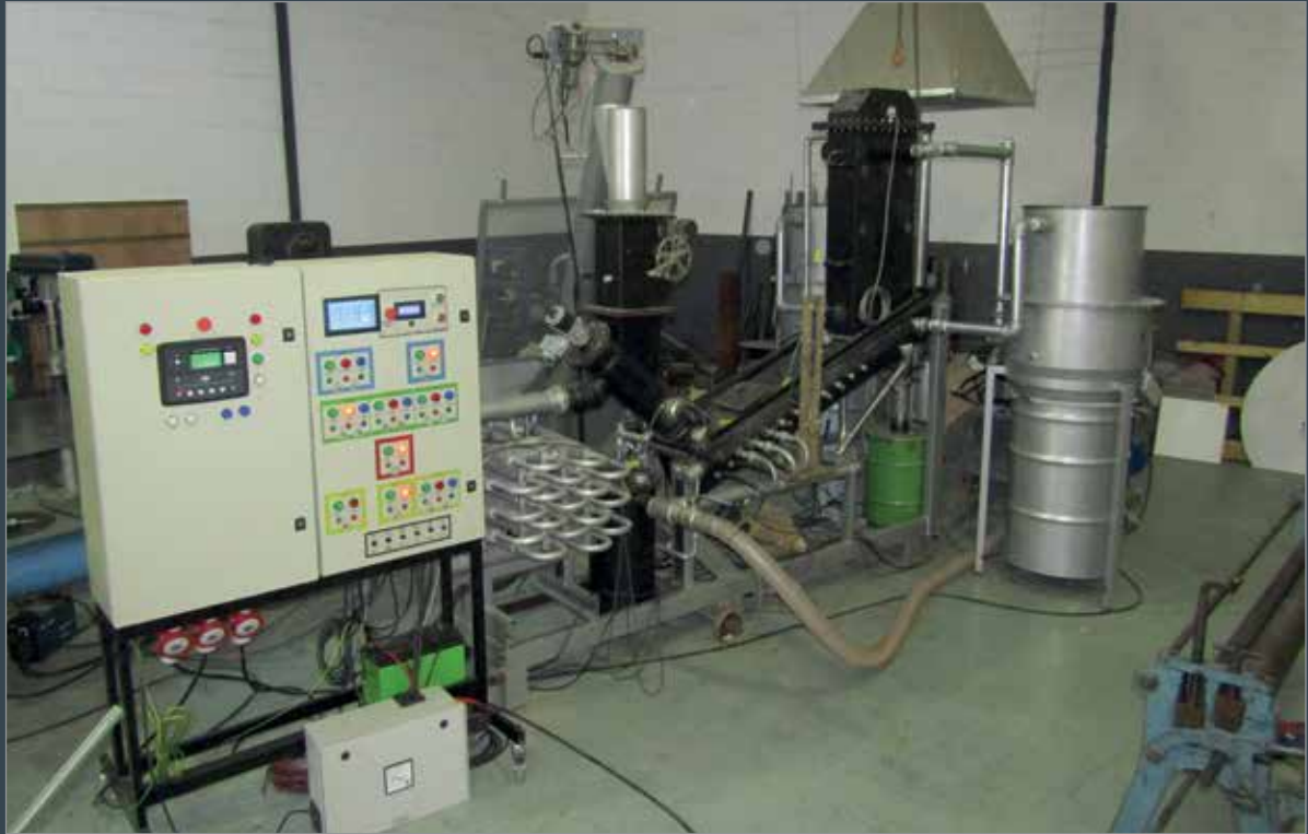
Figure 13: Pilot waste-to-energy gasifier plant
