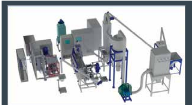
Figure 11: Schematic layout of the continuous supercritical fluid extraction plant
