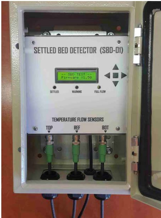
Settled Bed Detection Probe for the identification of slurry settlement on mines and oil sands industries.
