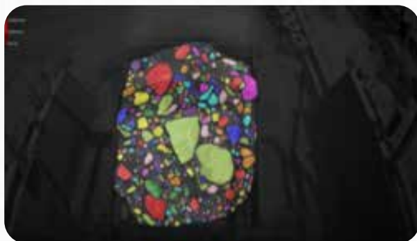
Figure 12: Stone Three's IntelliOre Truck technology for particle size segmentation
