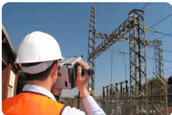
Figure 6: The Diagnostic Multi-camera in operation, showing how the camera enables the visualisation of corona discharge
