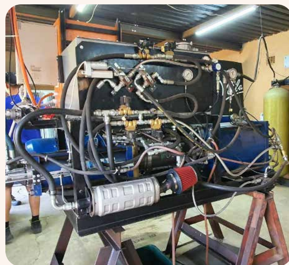
Figure 8: Compressed air energy storage system with storage containers
