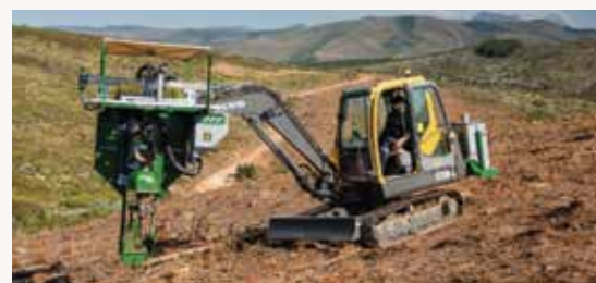
Figure 13: Field trials of the Novelquip ProPlant single head planter
