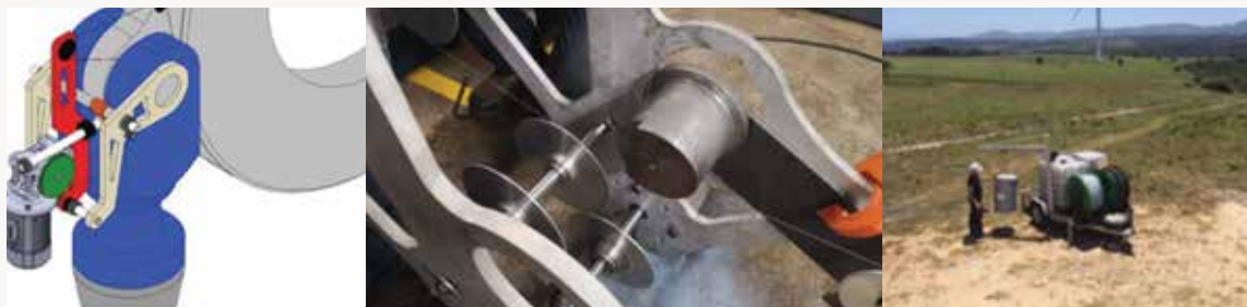
Figure 25: Concept design (left), prototype diamond wire cutter (centre), oil service equipment on site (right)
